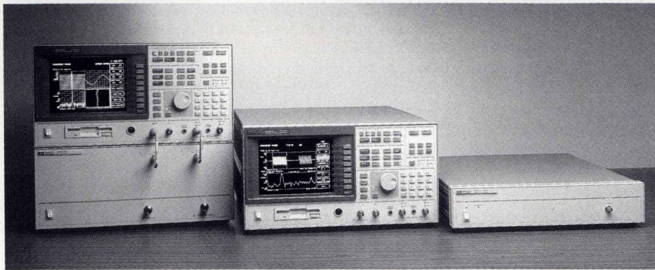
Fig. 1. The HP 89410A vector signal analyzer (center) is a 10-MHz baseband analyzer. It acts as the user interface, final digital IF, signal processor, and display section for the HP 894xxA family of analyzers. The HP 89440A RF section (bottom left) extends the analyzer's capabilities up to 1.8 GHz. The HP 89411A (right) is used with a higher-frequency analyzer to extend measurement coverage to frequency ranges above 1.8 GHz.
